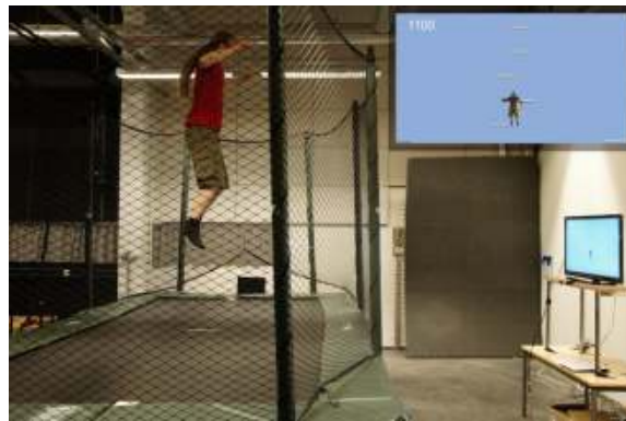
Figure 2. Test setup when participants were training with a game with exaggerated jumps (EJ). A screen shot from the TV is shown in the upper right corner.
