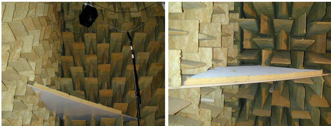
Figure 1: The measurement setup. A triangular chipboard covered with mineral wool is mounted between the wedges of anechoic chamber. In reported results, the microphone was positioned under the chipboard plate.
