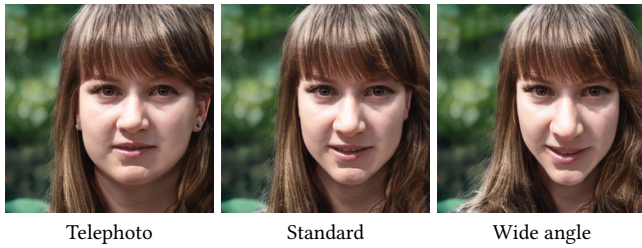
Figure 5: Changing the 3D camera’s field of view (equivalently, focal length) carries over to the rendered face but does not affect the background.
